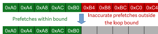
a DVR infers loop bounds at run-time to avoid over-prefetching large amounts of useless data.
