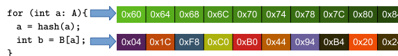
FIGURE 1. Vector Runahead (VR) detects striding access patterns and generates vector prefetches for the chain of instructions originating from the striding load, via an architecturally transparent transient runahead execution. This allows it to bring in complex data-dependent chains of memory accesses that are otherwise unpredictable.
